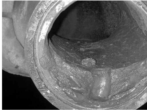
Fig. 6. Laminar flow settlement in paste fill pipe.
