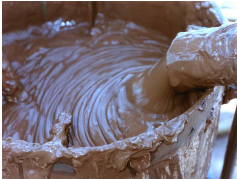
Figure 1: Viscous heavy mineral tailings slurry
