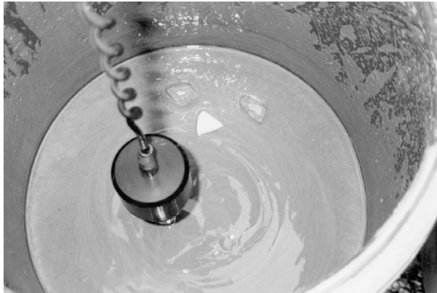
Figure 3: Particles supported by slurry yield stress (view looking down into a drum)
